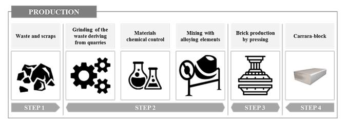
Fig. 1. Production of the "Carrara-block®"
