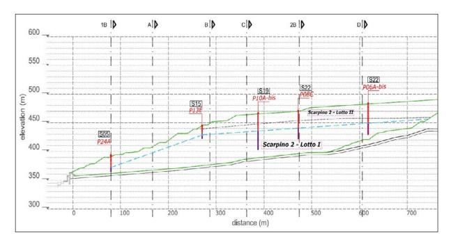
Fig. 7. Longitudinal section with the calculation scheme adopted to evaluate the liquid volume  $W_{S2}$  inside Scarpino 2. The landfill surface is shown in green line, the piezometric surface in dashed light blue, while the landfill bottom in black.
