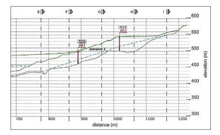
Fig. 5. Longitudinal section with the calculation scheme adopted to evaluate the liquid volume  $W_{S1}$  inside Scarpino 1. The landfill surface is shown in green line, the piezometric surface in dashed light blue, while the landfill bottom in black
