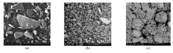
Fig. 4. ESEM micrographs of coarse (a), fine (b) CRT panel glass and quarz sand (c)
