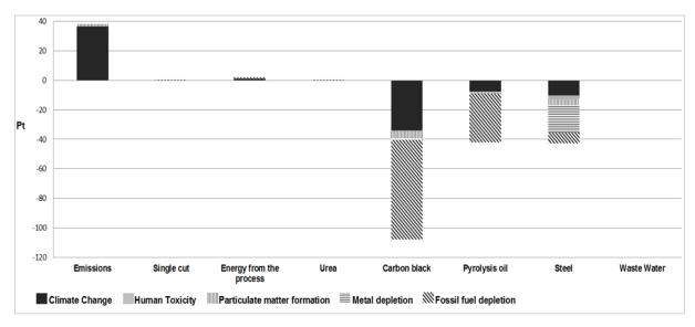
Fig. 2. Impacts of the pyrolysis process (Single Point, midpoint impact categories)
