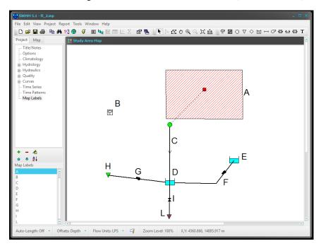
**Fig. 3.** Graphical representation of the SWMM model. The elements shown in the figure are: a subcathment (A), a rain gauge (B), a pipe (C), two storage units (D and E), two pumps (F and G), a weir (I), and two outfalls (L and H)
