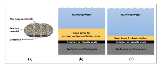
**Fig. 1.** (a) Reactive permeable mats (Zhang et al., 2016, modified), (b) active cap with sand protecting layer, (c) active cap with sand habitat layer
