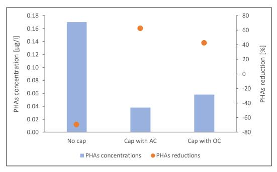
Fig. 4. PAHs concentrations in water after 20 days of capping test
