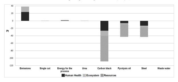
Fig. 3. Impacts of the pyrolysis process (Single Point, endpoint impact categories)
