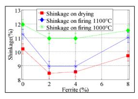
Fig. 5. Shrinkage of the slag-bricks extruded after drying and after firing
