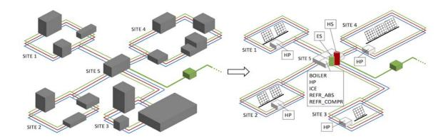
**Fig. 1.** From a generic district to the actual Campus: conceptual sketch. The algorithm is bounded to install each technology only in the pre-specified sites. Networks: blue = cooling, red = heating, green = electricity. The district is connected to the national electricity grid (green box). HP = heat pumps, ICE = internal combustion engine, REFR\_ABS = absorption refrigeration cycle, REFR\_COMPR = compression refrigeration cycle, ES = electrical storage, HS = heat storage
