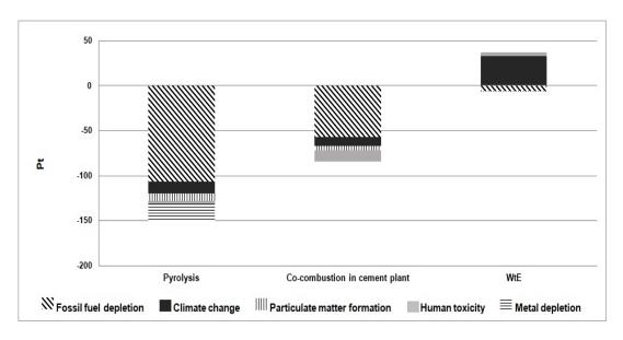
Fig. 5. Impact of the energy recovery processes (Single Point, midpoint impact categories)
