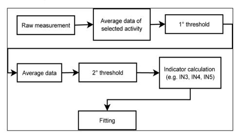
Fig. 2. Scheme of the data processing algorithm.
