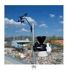
Fig. 2. PID (Corvus), Electronic nose (PEN3) (a) and meterological sensors (b)
