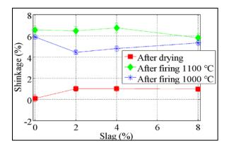
**Fig. 6**. Shrinkage of slag bricks pressed at 300 Bar after drying and after firing.
