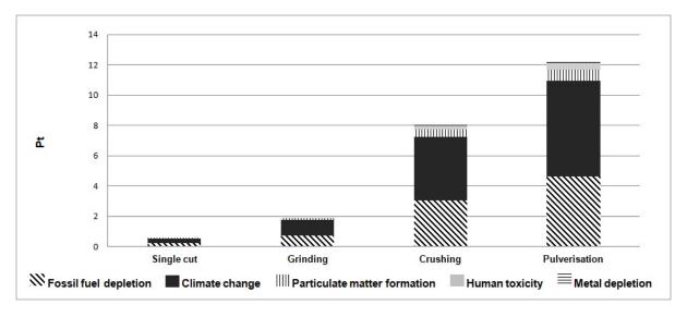
Fig. 4. Impacts of different pre-treatment process (Single Point, midpoint impact categories)
