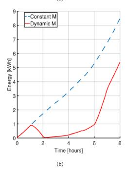
Fig. 8. (a) Trends of the PMV obtained by performing both the simulation cases;(b) energy consumption obtained by performing both control algorithms with a dynamic M and a constant M
