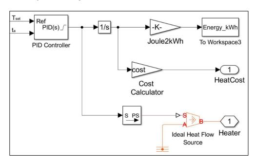
**Fig. 4.** PID controller applied to the simulation model.
