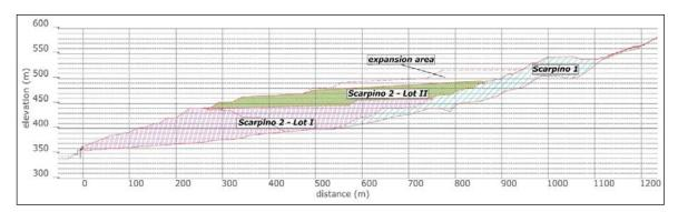
Fig. 2: Longitudinal section of the Scarpino valley with the main layers of the landfill
