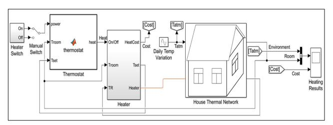
Fig. 5. Simulation model for the Heating house network.
