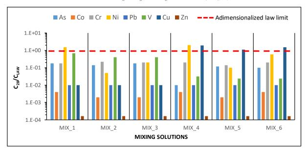
Fig. 5. Leaching at 28 days for each mix design and each heavy metal compared to law limit
