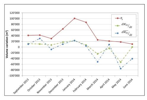
**Fig. 8.** Trends of the monthly variations in leachate volume within Scarpino 2 obtained by the hydrological balance equation (green line) and by the sections discretizing method (blue line) in comparison with the total rainfall volume (red line)
