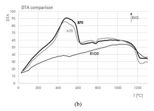
Fig. 8. TG (a) and DTA (b) analysis of the two mixtures prepared with a fixed percentage (30%) of pore forming agent, compared to R100, the mixture with only clay
