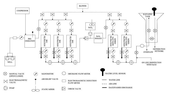
Fig. 4. Example of Mortara DWTP flow diagram
