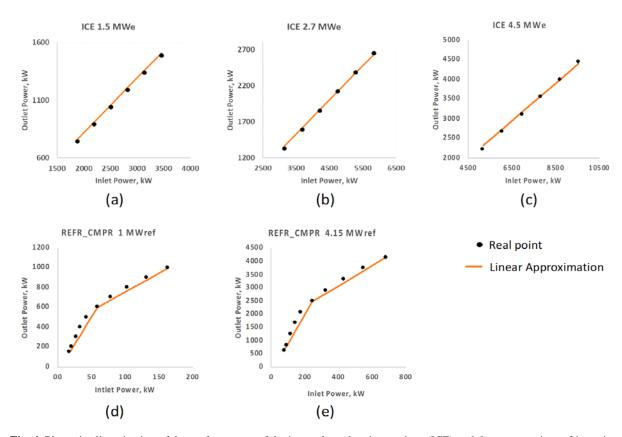
**Fig. 4.** Piecewise linearization of the performances of the internal combustion engines (ICE) and the compression refrigeration cycles (REFR\_CMPR): (a), (b), (c) are three relevant sizes for the ICEs in the "small" range and (d), (e) are two relevant sizes for the REFR\_CMPRs
