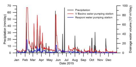
Fig. 2. Daily precipitation (mm) and daily drainage water volume  $(10^4 \, \text{m}^3)$  of "V Bacino" and "Rasponi" water pumping stations for the year 2015
