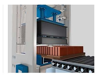
Fig. 3. High compression press used for the production of the "Ri-block®"
