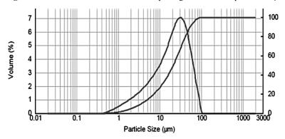
Fig. 2. Particle size distribution of fine glass CRT
