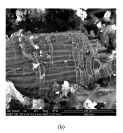
Fig. 2. Biochar particle structures at: 300x (a) and 600x (b) magnifications
