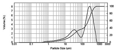
Fig.3. Quartz sand particle size distribution, peaks at 300 and  $35\mu m$
