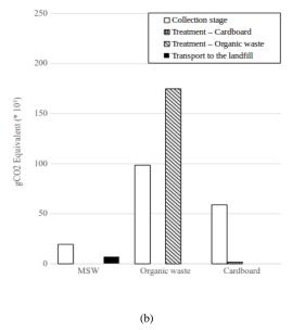
Fig. 4. Greenhouse gases emission in terms of gCO<sub>2</sub> for tonne of waste calculated for each waste stream
