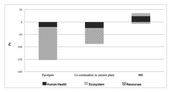
Fig. 6. Impacts of the energy recovery processes (Single Point, endpoint impact categories)
