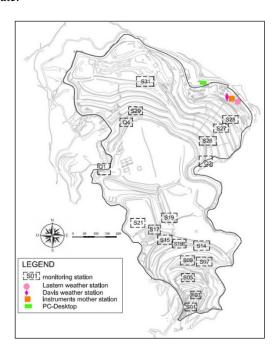
**Fig. 4.** Map of the installed instruments in the Scarpino landfill
