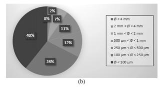
Fig. 6. Results of sieve analysis on biochar as received (a) and cyclone ashes as received (b)
