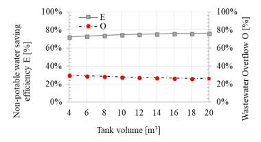
Fig. 9. Non-potable water saving efficiency -E and Overflow-O for different values of tank storage volume
