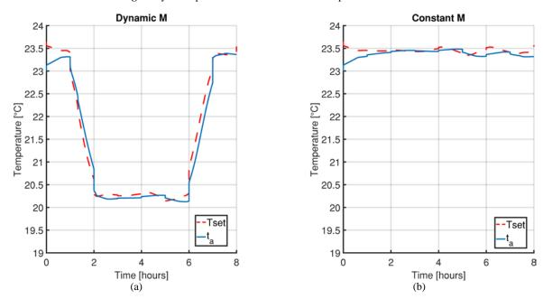
**Fig. 7.** Trends of the set-point temperatures and the air temperatures obtained by performing the two different controls: (a) with a dynamic profile of the metabolic rate; (b) with a constant value of the metabolic rate
