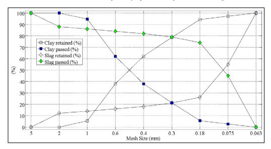
Fig. 1. Size distribution of clay and slag after 20 minutes of desegregation. Mesh size (mm) as reported on the used sieve
