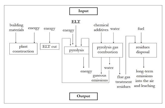
Fig. 1. Flow diagram of the pyrolysis plant studied
