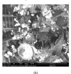
Fig. 3. Cyclone ashes particle structures at: 300x (a) and 600x (b) magnifications
