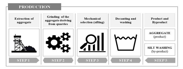
Fig. 1. Scheme of the process that generates silt washing
