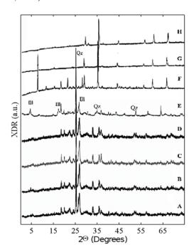
**Fig. 2.** XRD patterns of materials used to produce bricks and product after firing at 1000°C and 1100 °C. Curves E and F clay and cubilot slag as made; curves G, H slag after firing at 1000°C and 1100 °C respectively; curves A, Clay fired at 1100°C; curves B, C and D, mixtures clay slag after firing at 1100°C containing 2, 4, 8 % of slag respectively.
