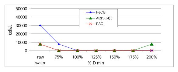
Fig. 2. Cyanobacteria cells concentration versus coagulant dose (indicated as percentage of the minimum dose) in the jar tests
