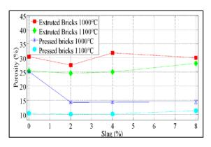
Fig. 7. Porosity of extruted and pressed bricks after firing at 1000 and 1100°C for 120 min. (UNI-EN 8942)
