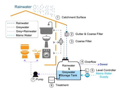
Fig. 1. Scheme of a hybrid system in which the rainwater and the greywater are combined into a single supply source
