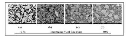
Fig. 5. ESEM micrographs of glass samples: (a) 0%; (b) 10%; (c) 20%; (d) 30% of fine glass
