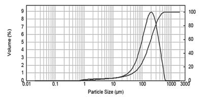
Fig. 1. Particle size distribution coarse CRT panel glass, is show a peak at 200μm
