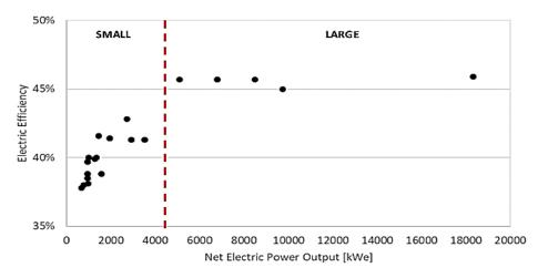
Fig. 3. Classification of engines based on the correlation between electric efficiency and net electric power output
