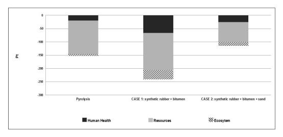
Fig. 8. Impacts of the material recovery processes (Single Point, endpoint impact categories)
