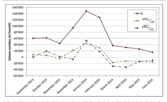
**Fig. 6**. Trends of the monthly variations in leachate volume within Scarpino 1 obtained by the hydrological balance Equation (green line) and by the section discretizing method (blue line) in comparison with the total precipitation volume (red line)
