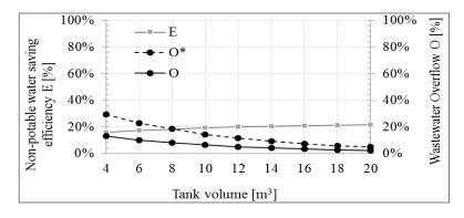
**Fig. 10.** Rainwater harvesting system: non-potable water saving efficiency -E and Overflow-O for different values of tank storage volume
