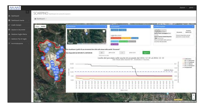
**Fig. 3.** Dashboard visualization of the monitoring system (left). A zoom, when you click on a station (in this example, S01), of the leachate level data (right) measured by a water level sensor
