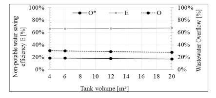
Fig. 11. Greywater reusing system: non-potable water saving efficiency -E and Overflow-O for different values of tank storage volume
