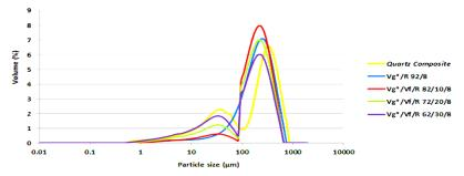
Fig. 6. Comparison particle size distribution of samples glass and quartz composite
