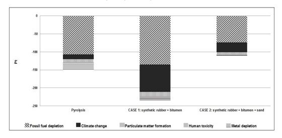
Fig. 7. Impacts of the material recovery processes (Single Point, midpoint impact categories)
