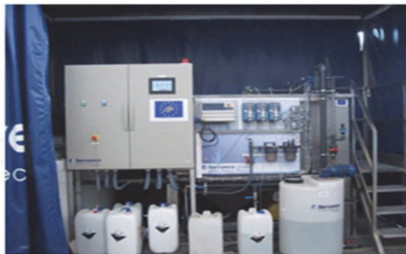
Fig. 2. Coagulation/flocculation pilot unit
